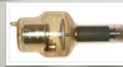
Rotating anode X-ray tube
