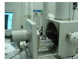
SEM opened sample chamber
