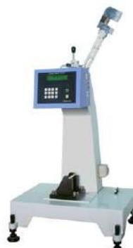
**Impact energy** = The loss of the hammer's potential energy (J)
