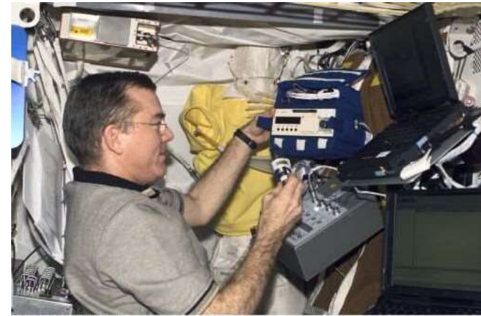
An american astronaut uses the TLD dosimeter „Pille” produced by KFKI Budapest (Photo: NASA ISS002E7814)
