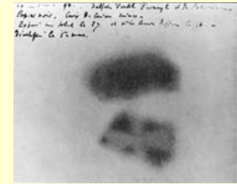
Image of Becquerel's photographic plate which has been fogged by exposure to radiation from a uranium salt. The shadow of a metal Maltese Cross placed between the plate and the uranium salt is clearly visible. (1896)
