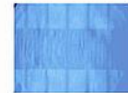
blurred image of the optical grating (limiting case, 10 μm lines are just not visible)
