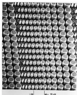
Figure 3. Scanning electron micrograph of a 2 dimensional VCSEL array. Photo by Axel Scherer, Courtesy of Picolight, Inc., Boulder, CO.
