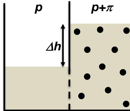
Hydrostatic pressure difference
