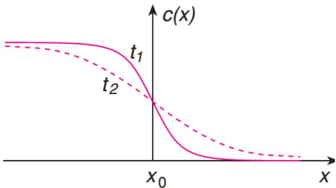
$$c(t + \Delta t) = c(t) + D \cdot \Delta t \cdot \frac{\Delta \left( \frac{\Delta c}{\Delta x} \right)}{\Delta x}$$
