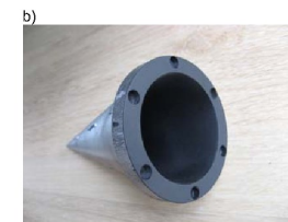
Fig. 2. Geometry of the cone radiator with its computational perfectivity (a) and the manufactured cone (b)
