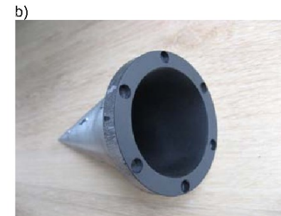
Fig. 2 Geometry of the cone radiator with its computational geometry (a) and the manufactured cone (b)
