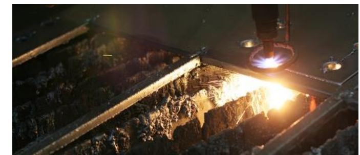
CO 2 laser (cutting a metal sheet)
