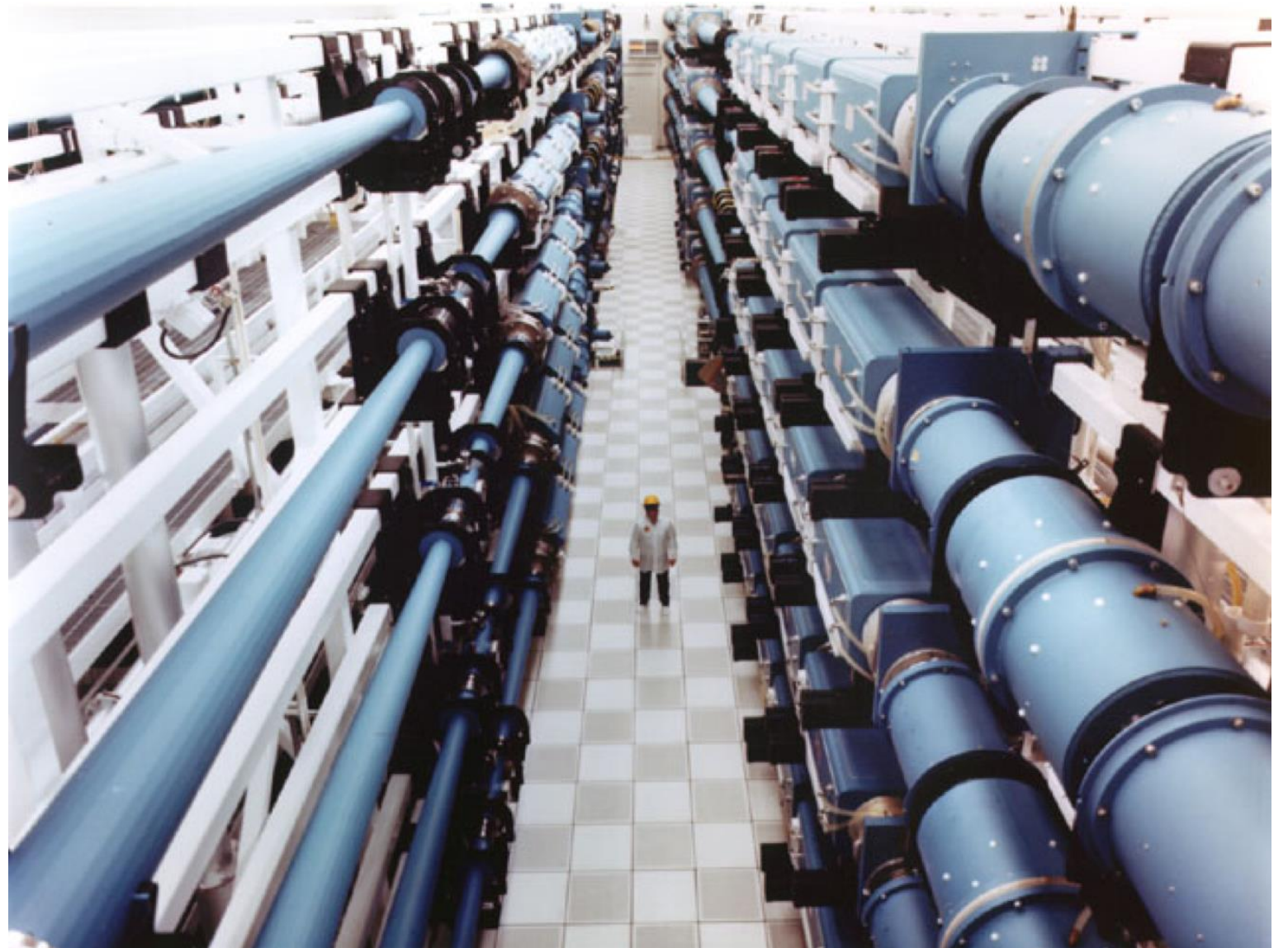
Terawatt NOVA laser - Lawrence Livermore Laboratories Size of a football field
