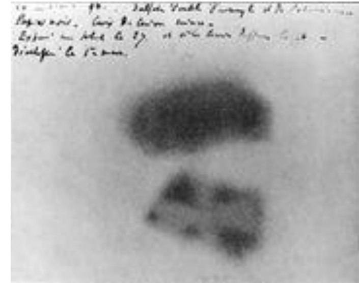
Image of Becquerel's photographic plate which has been fogged by exposure to radiation from an uranium salt. The shadow of a metal Maltese Cross placed between the plate and the uranium salt is clearly visible. (1896)
