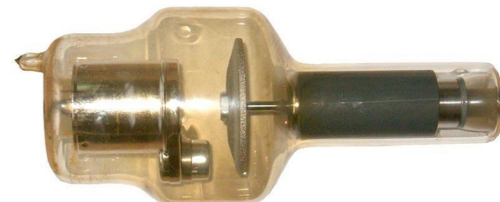
Rotating-anode X-ray tube. Anode rotation is used for cooling.
