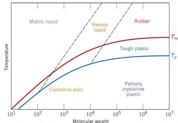
**T<sub>m</sub>** is the temperature at which crystalline domains lose their structure, or melt.
