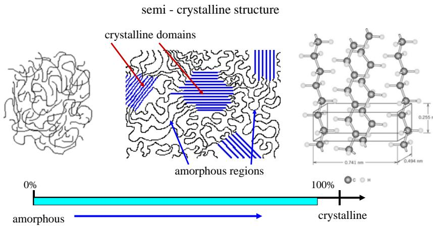
factors influencing the degree of crystallinity: temperature, type of the monomer, **chain length, chain branching, interchain bonding**
