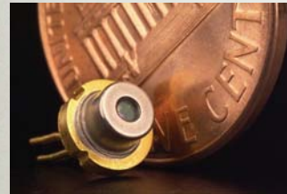
5 mW diode laser few mms
