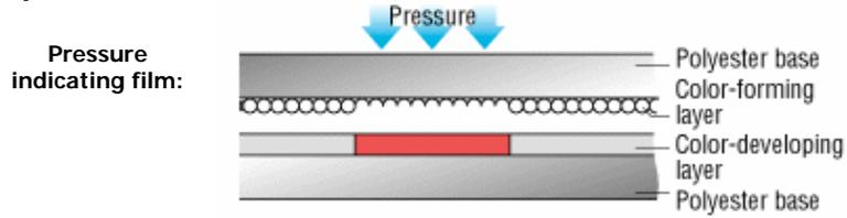
micro-encapsulated color forming and developing material
