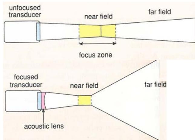
Focusing increases the divergence of the beam in the far field regime and reduces the depth sharpness.
