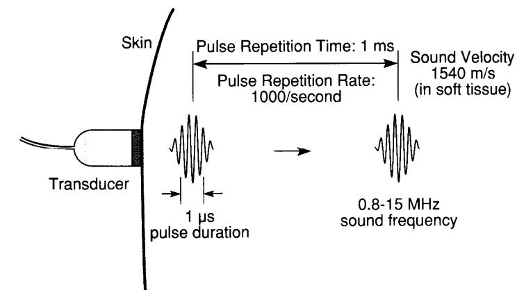
$J$  understood in the pulse with  $\Delta t \sim 1 \mu\text{s}$  and  $1 \text{ ms}$  pause
