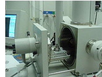
SEM opened sample chamber
