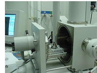
SEM opened sample chamber
