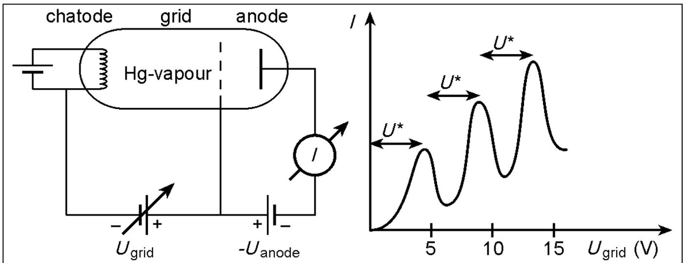
anode is reached only by those electrons that have enough kinetic energy  $E_k$  to overcome the work  $eU_{\text{anode}}$ :  $E_k \geq eU_{\text{anode}}$
