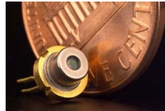
5 mW diode laser few mms
