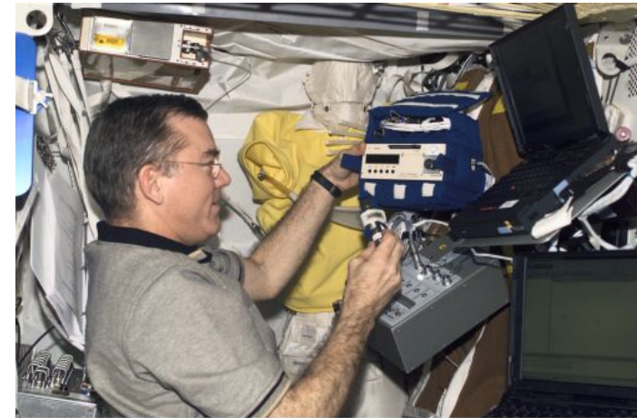
An american astronaut uses the TLD dosimeter „Pille” produced by KFKI (Photo: NASA ISS002E7814)
