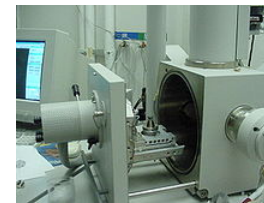
SEM opened sample chamber
