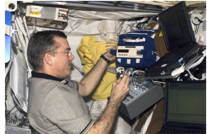
An american astronaut uses the TLD dosimeter „Pille” produced by KFKI (Photo: NASA ISS002E7814)
