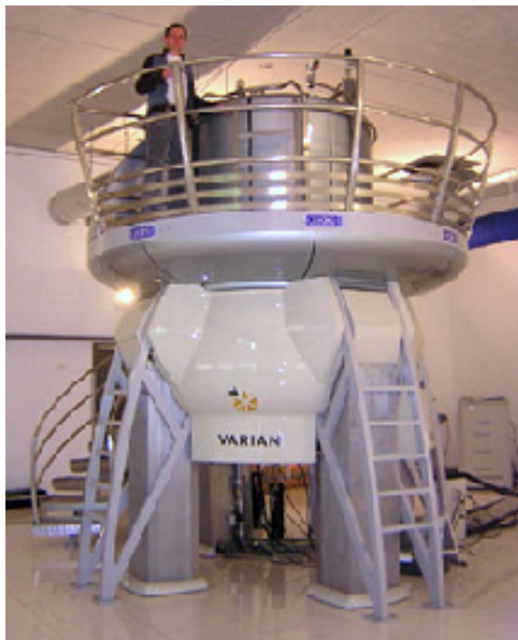
900 MHz NMR, 21.1 T magnet (cooled with liquied He; spectral resolution proportional to magnetic field)
