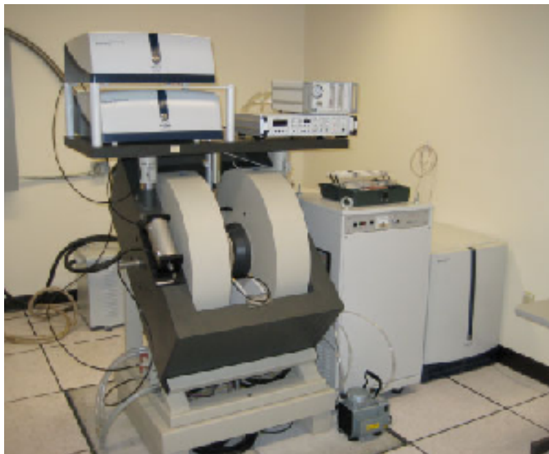
ESR spectrometer (smaller magnet (hence magnetic field), higher-frequency EM radiation (microwave))
