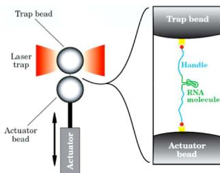
force-guided unfolding of viral RNA using laser tweezers
