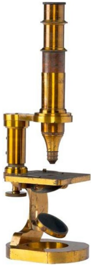
Microscope by Carl Zeiss (1879) with optics by Abbe
