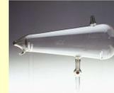
Glass tube with two electrodes in vacuum or in low pressure gas
