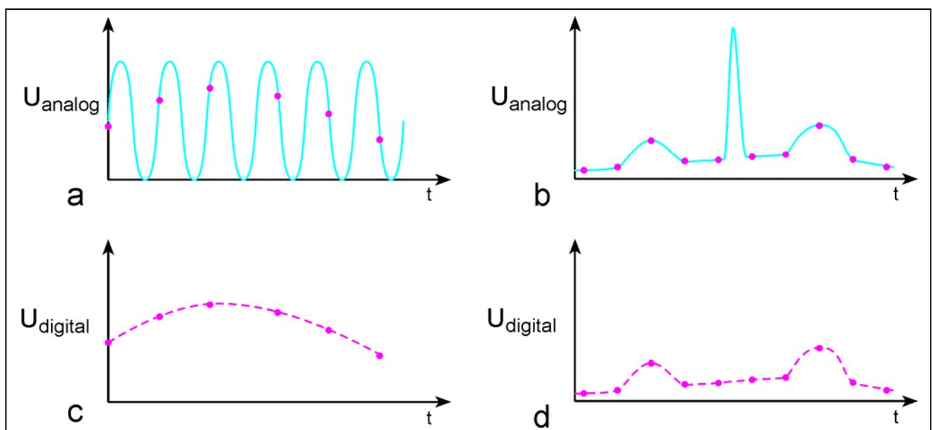
3. frequency of the sampling (Usually, the input voltage changes continuously, so the converter always measures its value after a certain period of time (it samples the signal). It is crucial that the sampling frequency is adjusted to the signal.) (**Bad sampling!**)
