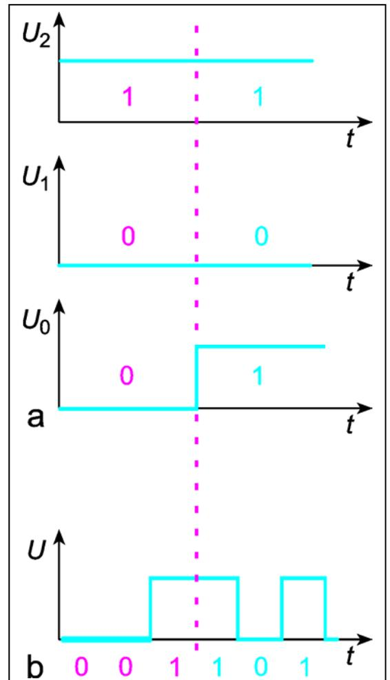
For example, 3 parallel BD voltage signals have altogether  $2^3 = 8$  different configurations, hence we can display numbers from 0 to 7.
