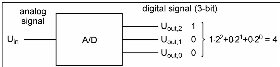
Important parameters of the A/D converter:
