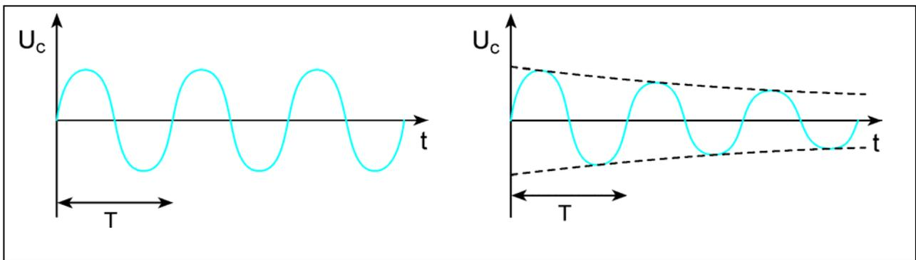
The voltage on the capacitor of an ideal and a realistic oscillator is constant amplitude and damped sinusoidal, respectively
