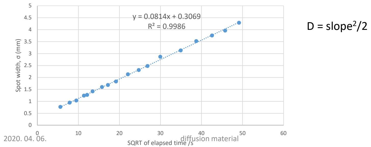
The average distance covered by a particle can be calculated from the random walk model
