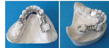
metallic framework of a partial removable dental prostheses (PRDPs) processed by laser melting
