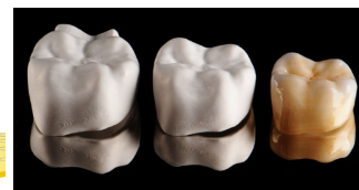
„green body“ „white body“ finished crown cross-linked organic binder and zirconia particles cleansing, thermal post-processing (1000 °C) after the stain/glaze firing (770 °C)
