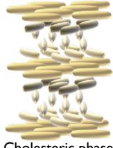
Cholesteric phase (nematic order in different planes; special case: twisted nematic phase - pitch affects color)
