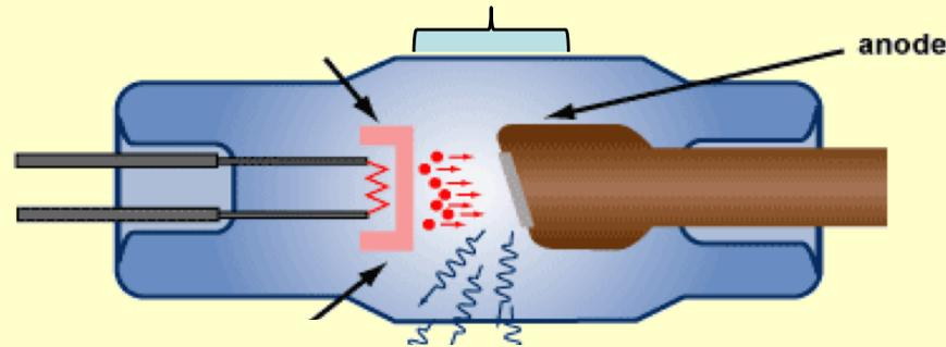
Anode: higher atomic numbers and higher melting points needed.
