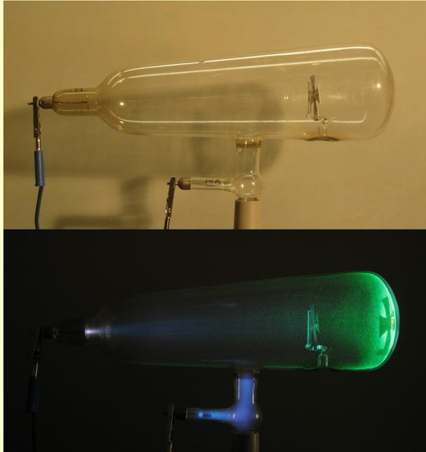
William Crookes' tube: electrical discharge tube with partial vacuum
