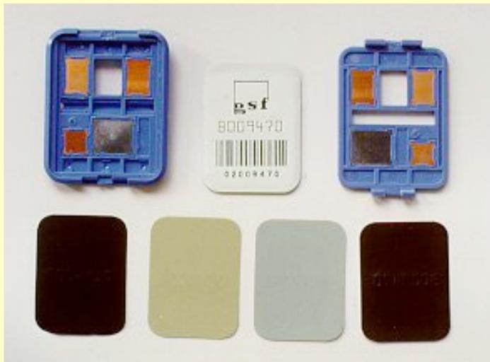
It measures darkening of the developed photographic film that was exposed to ionizing radiation.
