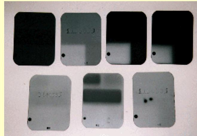
Darkening of the developed photographic film is proportional to the dose rate of the ionizing radiation and to the irradiation time.
