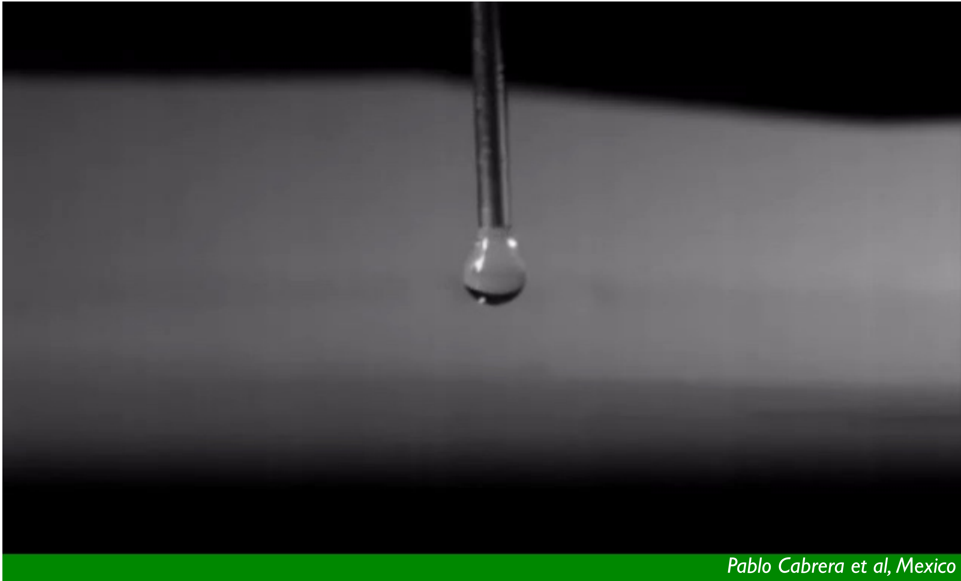
Persisting water droplets on vibrating water surface
