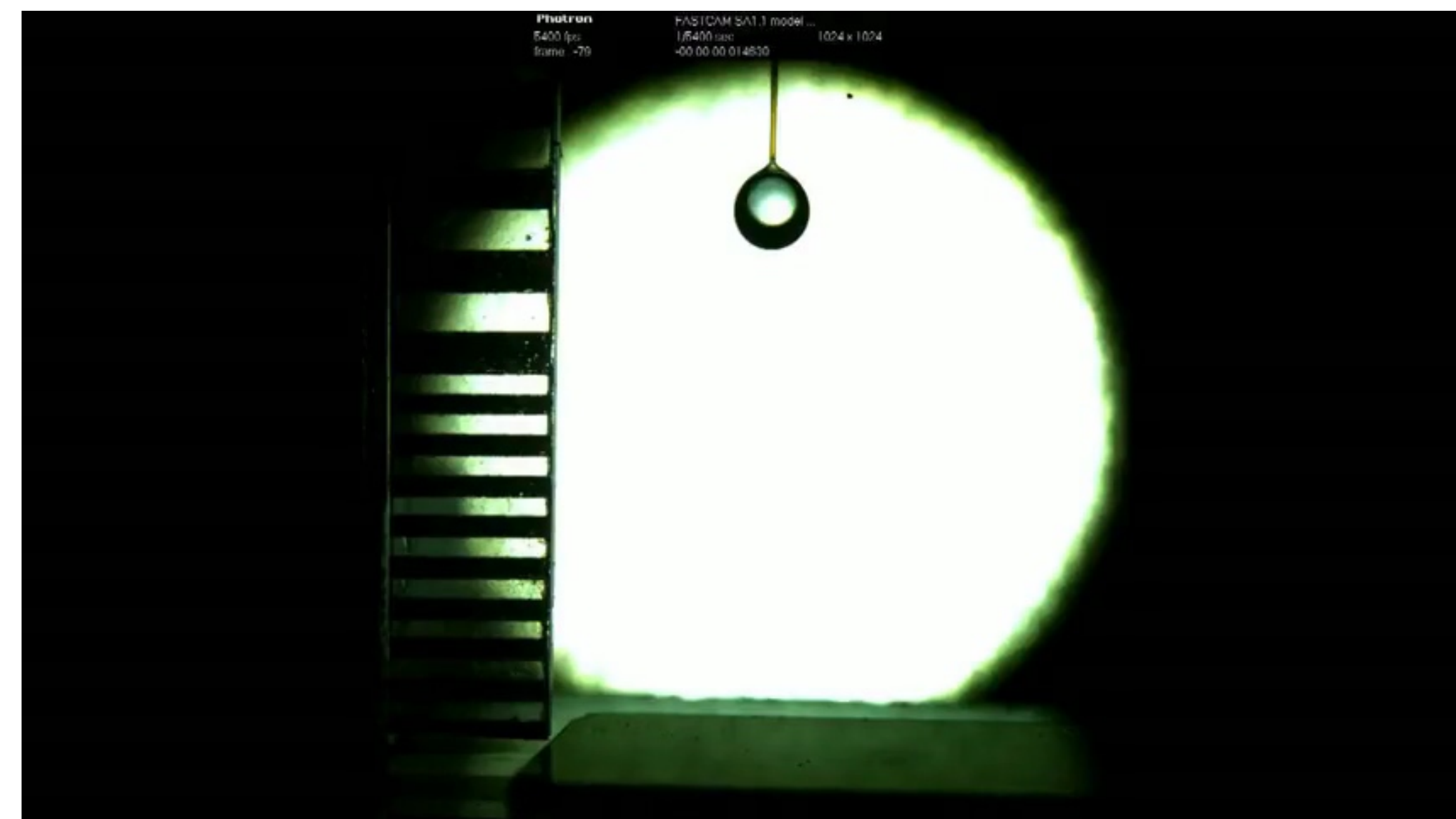
Persisting droplet on a superhydrophobic surface
