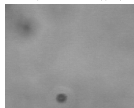
3 μm latex (polystyrene) microspheres in the optical trap
