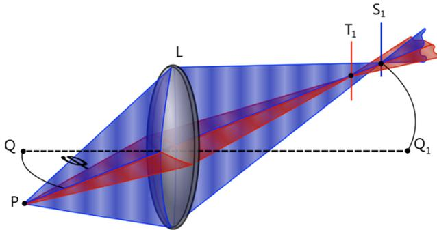
Correction with cylindrical lens.
