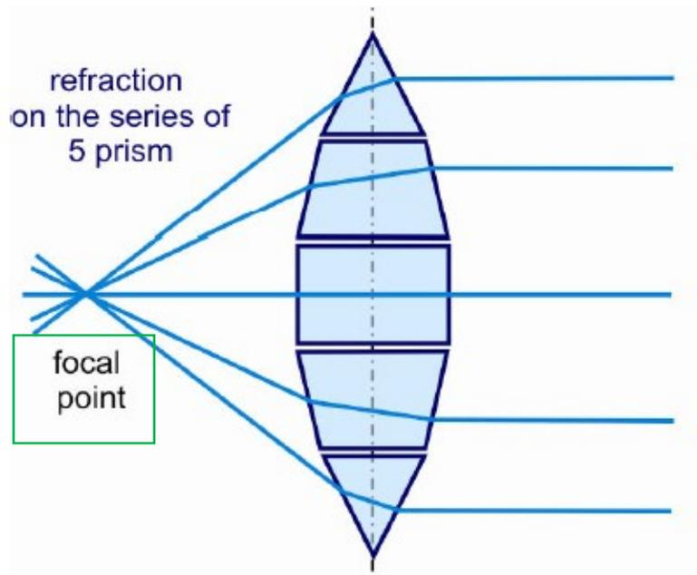
with a suitable arrangement rays originating (or coming) **out of one point** will become parallel, and vica versa.
