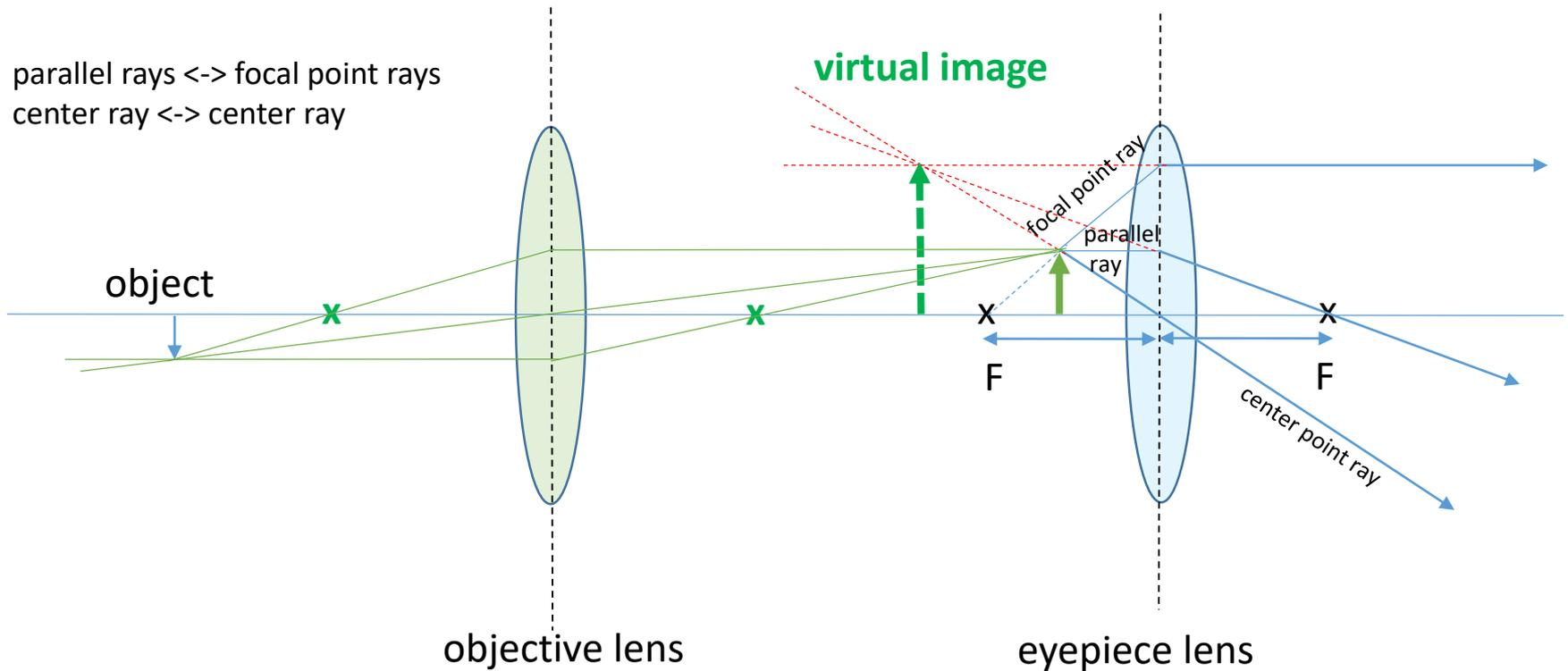
The microscope can be set to see the virtual image at the reading distance of 25 cm, but also to accommodate to infinity (like looking at the sky). The magnification will be different.
