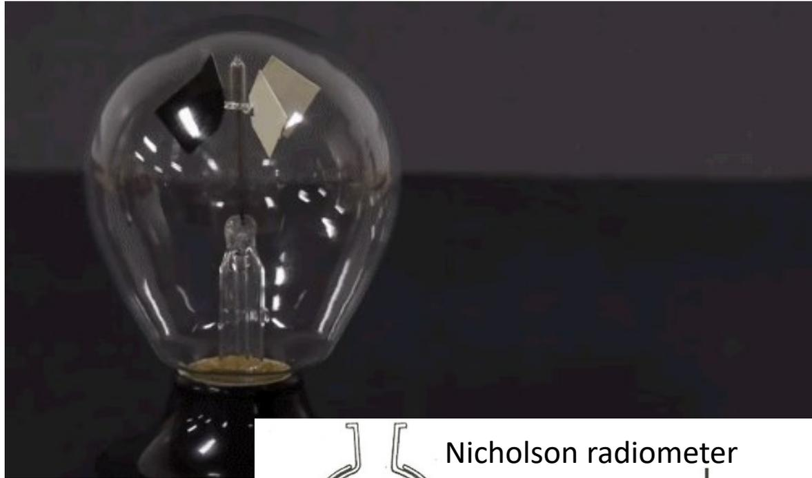
at refraction or reflection the wave exerts a very small force on the object. But if the object is very small ( $\mu\text{m}$ -sized bead under the microscope) or an easy to move almost frictionless object in vacuum then the force is enough to make them move (Nicholson radiometer)!
