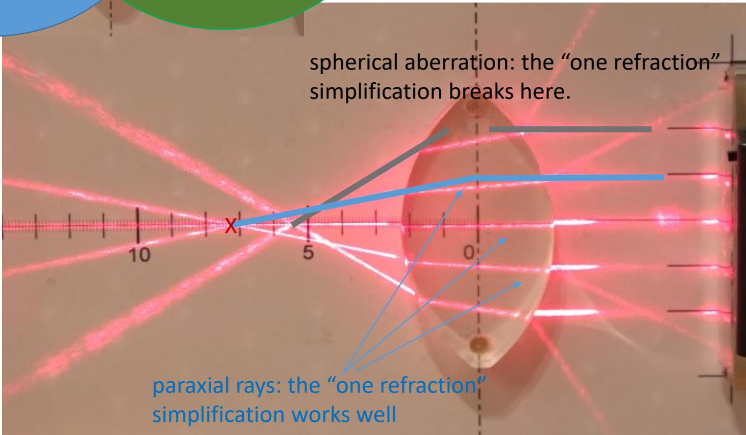
paraxial rays: the “one refraction”
