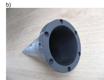
Fig. 2. Geometry of the cone radiator with its computational emissivity a) and the manufactured cone b)
