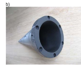
Fig. 2. Geometry of the cone radiator with its computational perfectivity \epsilon and the manufactured one by
