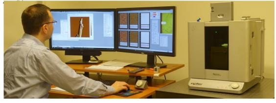
**Molecular Force Spectrometer** With the Molecular Force Probe force spectra of mechanically manipulated single molecules may be rapidly collected.
