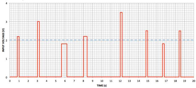
20. The graph below shows the input voltage of a bistable multivibrator as function of time. The voltage threshold of the multivibrator is 2 V and it is sensitive only for the trailing edge of the input voltage signal. The voltage of its active state is 2.5 V while that of its passive state is 0 V, the multivibrator is initially in the passive state. Plot the output voltage as function of time.
