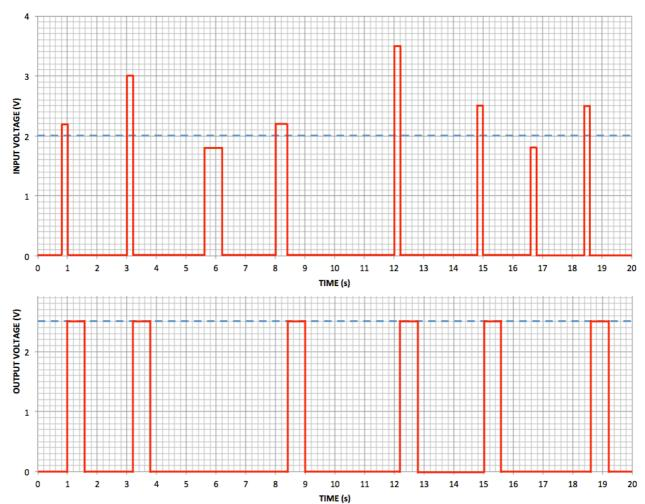
20. To the trailing edge of every over-the-threshold voltage pulse input (at 1 s; 3.2 s; 8.4 s; 12.2; 15 s; and 18.6 s) belongs a transition between the active and passive states. The trailing edges at 6.2 s and 16.8 s belong to below-the-threshold voltage pulses so they will not trigger a response.
